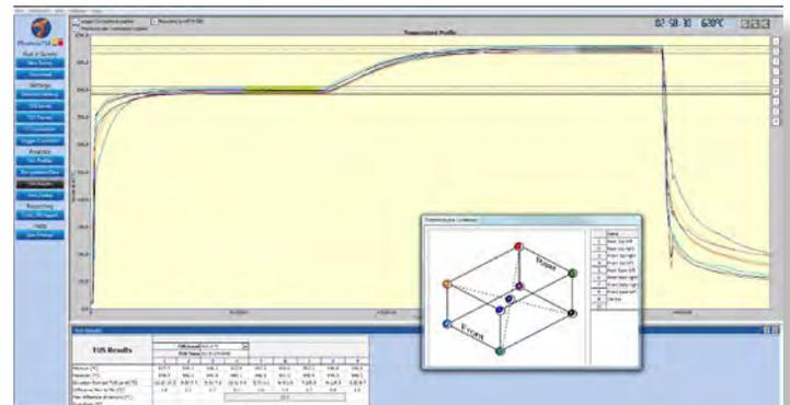
A separate software package, "Thermal View Survey" is available for surveying furnaces to industry requirements. Featuring thermocouple and data logger correction factors, user defined TUS levels and tolerances, View Frame analysis, over shoot search, data import / export, printed report. Contact us for a demo version!
