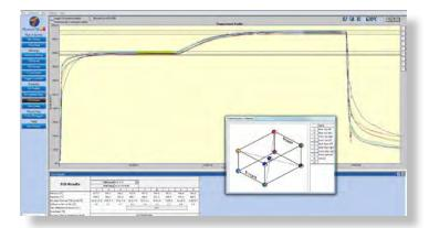
A seperate software package, "Thermal View Survey" is available for surveying furnaces to industry requirements. Featuring thermocouple and data logger correction factors, user defined TUS leves and tolerances, View Frame anaylsis, over shoot search, data import / export, printed report. Contact us for a demo version!
